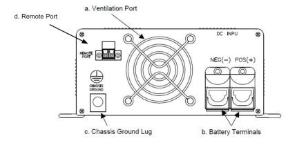
**Warning!** Operation of the inverter without a proper ground connection may result in an electrical safety hazard.
